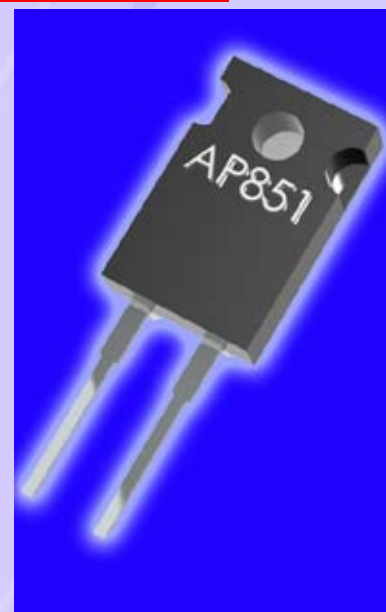
AP851 TO220 50 Watts (Tab Temp Max 25°C) 1R 10K \pm 0.5\% , \pm 1\% , \pm 5\% , \pm 10\% \pm 50 to \pm 300\text{ppm}/^\circ\text{C} (re ohmic value) 420Vdc or \sqrt{P,R} 18000 Vdc (60 secs)
